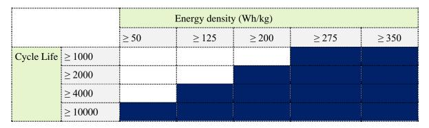
Both the performance parameters i.e., energy density and cycle life have to be demonstrated at same level of Depth-of-Discharge.
